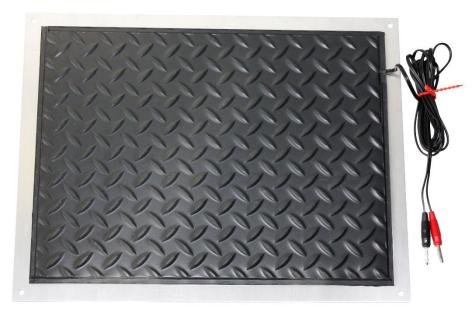
The time from leaving the mat until landing on the mat is measured by the timing device TIMY3. From the measured "time in the air", the timing device is calculating the height of the jump.
