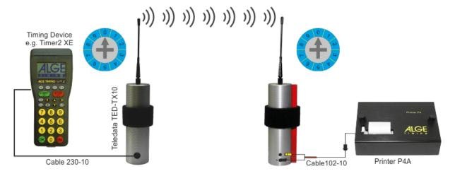
If the output "RS232" is used by a timing device, you must use cable 060-10 for the TED-TX.
