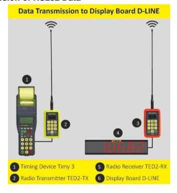
The data transmission of RS232 data is designed for large display data. However, any other data can also be transmitted. The baud rate on the transmitter is set to 2400 baud. The receiver automatically recognizes whether it is a matter of times or dates. Times are automatically output at 9600 baud, data at 2400 baud.
