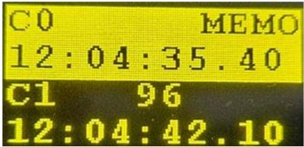
With the "memo" menu you can switch to memo-mode. This mode is used if it is not clear which competitor is next, e.g. at the finish area when you cannot see the competitor come closer. The bib number at the first time blinks. You can confirm the given bib with  $\longleftarrow$  or you can enter
