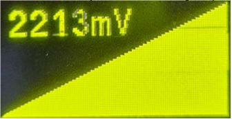
The higher this value, the better the reception. If no field strength is displayed on the receiver, then it is out of range. Stable reception is possible from around 1200mV. You can cancel this field strength test at any time with "ESC".
