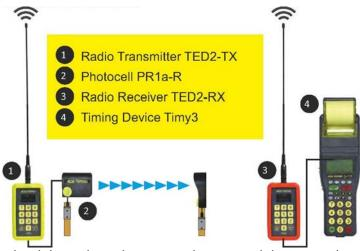
The times are transmitted three times in a row using a special process (patent pending). This serves to ensure transmission security and to prevent deletions. Depending on the channel, the transmission can take up to 2.1 seconds. If the first transmission is successful, the time pulse can be output as a pulse by the receiver with a delay of exactly 0.1s. However, since the ID-number is transmitted with the TED2 system, we recommend connecting the Timy2 or Timy3 using cable 319-03 or 327-02.
