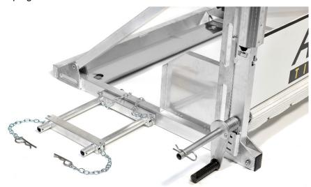
Push the two SSD1 together and fix them with the spring pin
