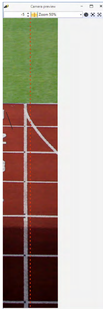
Picture after levelling the camera vertically. Use the line shifting or gearhead to move the scan line to the correct place.
