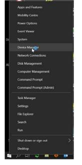
The RS485 Port from the USB-WTN is Listed in your Device Manager as a simple USB-Serial Port. There are 2 Ports on the USB-WTN, normally the lower Port-Number is the RS485 connection to the WTN and the higher one is the RS232 connection. You have to enter the RS485 Port-Number in the Wtn Settings of the Sync&Dive Software!
