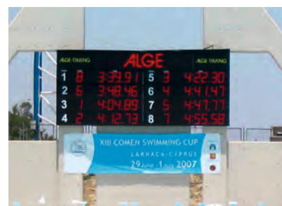
seven segment LED display board with LED matrix display board D-RTNM (top)
