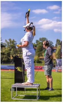
The SJ2 false start system does not require any operation during the start process. The measurements are made automatically. Each start sensor collects the start data and transmits them to the Notebook in the Start Judge Cart, which is connected via a USB cable.
