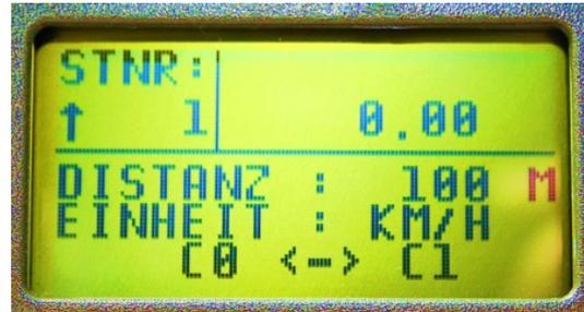
If the start-photocell is triggered out, the display will show instead of “0.00” a dotted line. Timy will calculate from the adjusted distance and min. speed, how long one cycle will take at maximum. If this time will be crossed, the display will show “0.00” and is ready for the next measurement.
