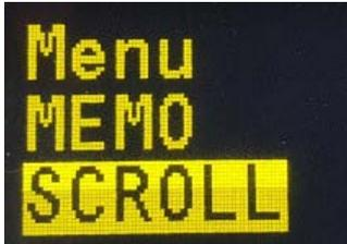
Open the selection menu with the ESC button. Press ESC once again for returning to the main screen. Use the arrow buttons ('2' for scroll up, '8' for scroll down) to choose the menu item. Press
