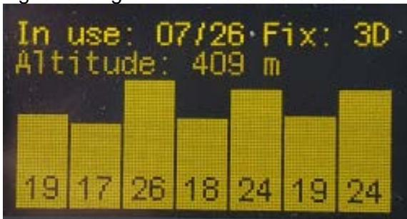
The GPS receiver uses GPS, GLONASS and GALILEO satellites.
