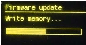
After finishing the download, press the ON/ESC button to restart the device.
