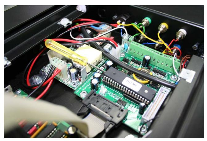
For the right side use tool n. 4 and lift the processor out of the socket
