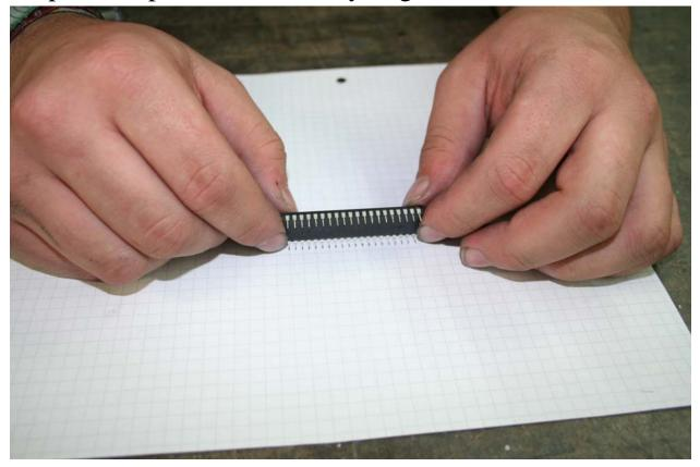
For this give the processor parallel to an plane ground. Now bend the pins parallel too the ground so that the distance are less then before. You must make this until then the processor falls into place of the socket. Push the processor, with the indentation for the first pin on the right side, into the socket. When you have made the last step correct, you can push the processor with bouth hands planar into the socket
