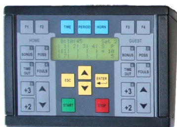
control terminal D-CKN
