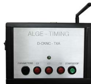
Console D-CKNC-TXA to control the Countdown-Display Board
