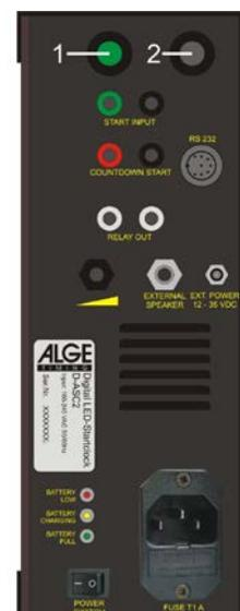
**b) External push-button connected at red and black banana socket (4):**
