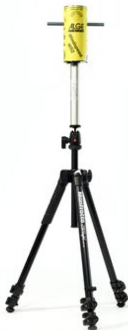
The ALGE-TIMING Windspeed WS2 works with a calorimetric mass flow sensor, which allows fast and accurate wind measurement.
